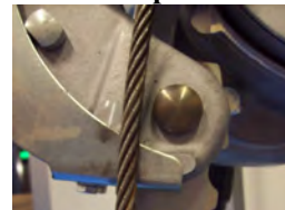
Locked Stirrup Bar Position
