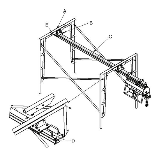
**Figure 5.5**I-Beam Suspension Brackets
