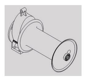
**Figure 3.2**Transmission and Drum
