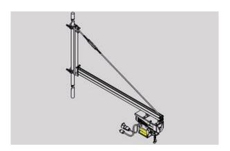
**Figure 3.9**Sliding Trolley Shown with Beta Lite Hoist
