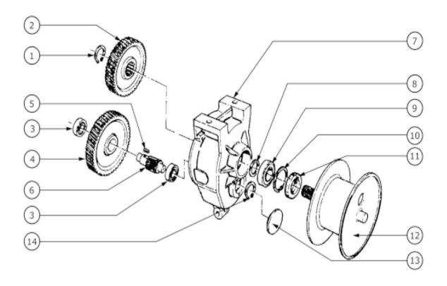
**Figure 10.2**Transmission and Drum
