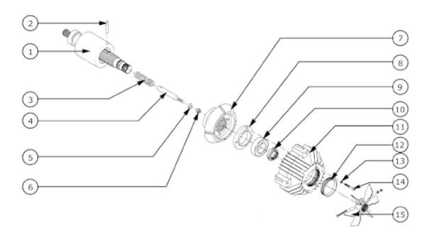
**Figure 7.1**Conical Brake Exploded View
