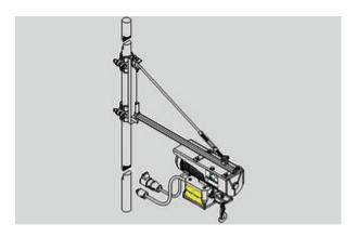
**Figure 3.7**Vertical Post Shown with Beta Lite Hoist
