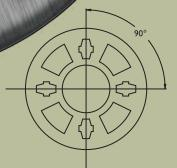
The Universal System Scaffold Rosette provides total flexibility to lock in any angle plus quickly and accurately align at 90° angles using the keyhole positions. Each Rosette can have up to eight connections at one time.
