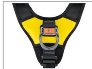
Fall indicator on the dorsal attachment point: a red strap appears on the dorsal attachment point after a fall to indicate that the harness should be retired.
