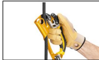
The safety catch allows the handled rope clamp to be installed or removed anywhere on the rope with one hand. It is easily manipulated, even with gloves.
