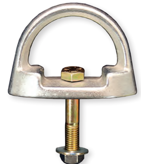
1550 D-bolt anchor (designed for anchoring into steel structure) Designed to prevent roll-out of snaphooks Grade 8, 1/2" bolt, washer, and lock nut 1 3/4" maximum steel thickness
