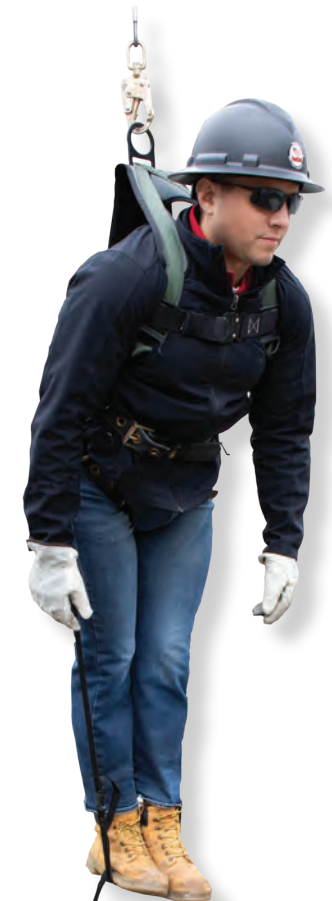
STEP 4. Stand vertical in web loop to relieve harness tension
