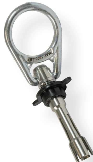
1772 3/4" portable/reusable concrete hole anchor Rated to 5,000 lbs Use for vertical and overhead concrete Swiveling action prevents tangles
