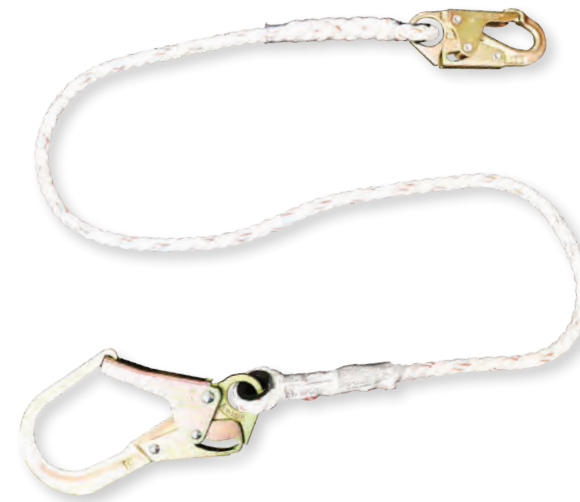
404 6' polyblend rope lanyard #Z74 locking snaphook at one end #Z136 rebar snaphook (2 1/2" opening other end)
