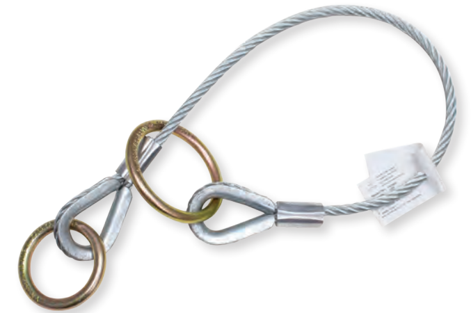
1600VC Cable tie-off adapter (pass-thru style) 5/16" vinyl coated cable 4" O-ring one end, 3" O-ring opposite end
