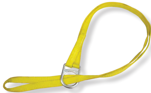
1122HD Web scaffold/pipe choker 1" 9800 lb. web, chocker style, 22" long Attaches to anchors up to 3" diameter
