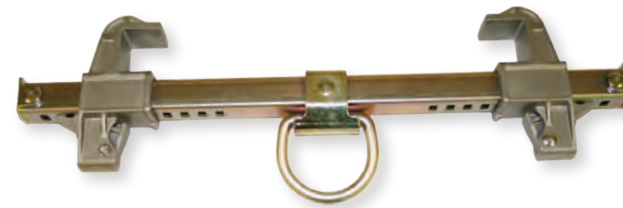
1700 Adjustable sliding beam anchor Fits flanges 3 1/2" to 12" wide, up to 1 1/4" thick Usable on top or bottom of I-beam Center D-Ring for smoother slide
