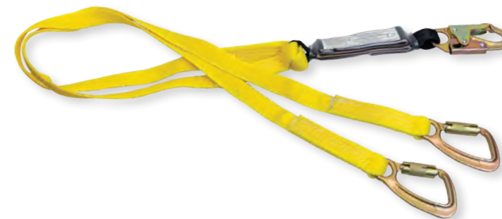
446AW Dual leg (100% tie off) #Z74 locking snaphook one end #63 (3/4" opening) auto locking snaphook other end Pack style shock absorber
