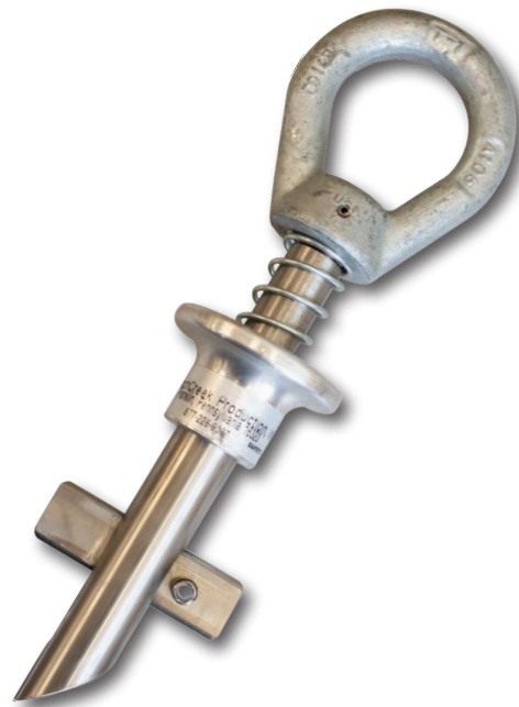
1769 Steel toggle anchor (Installs into pre-drilled hole) Fits 3/4"- 1 1/4" pre-drilled holes 1" maximum steel thickness
