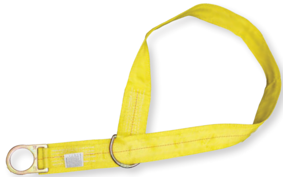
1300-WP Web tie-off adapter 1 3/4" web, 3" wide polyester wear pad 3" D-ring one end, 2" D-ring opposite end
