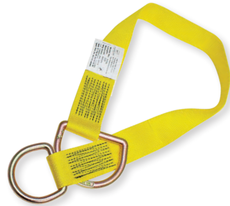
1300 Web tie-off adapter 1 3/4" web 3" D-ring one end, 2" D-ring opposite end
