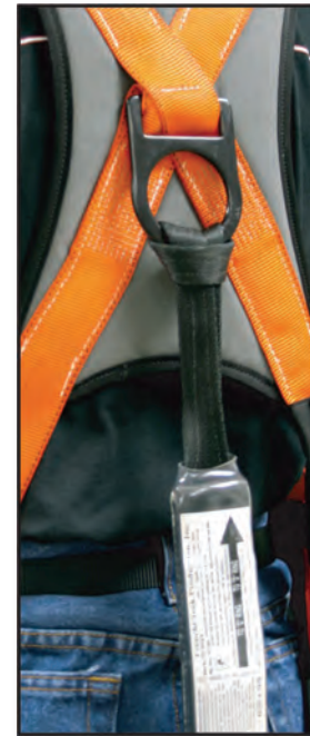
Choke-Loop 1 Pack-style shock absorber Looped End
