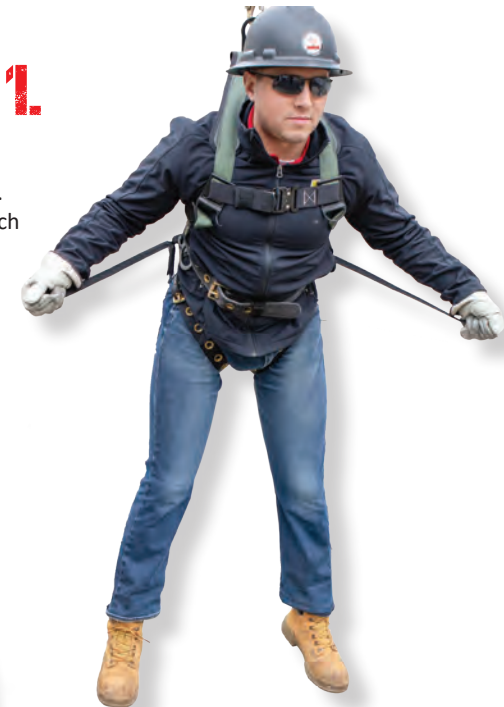
STEP 2. Adjust to appropriate length and buckle straps together
