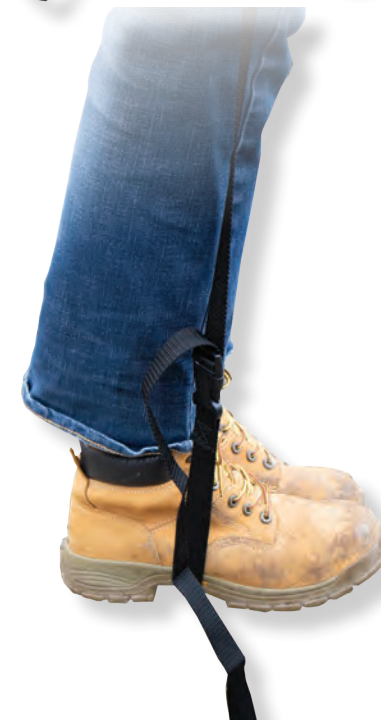
STEP 3. Step into web loop with both feet
