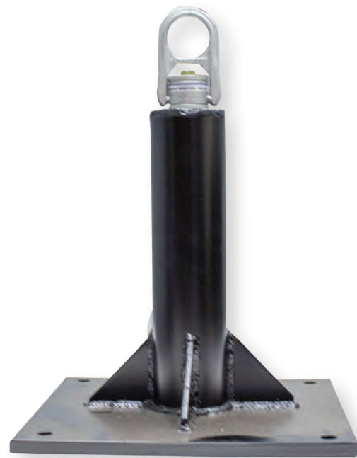
1760-12S 12" Anchor Post (Bolts to steel surfaces) Includes four 1/2"-13X 3" length grade 5 bolts, nuts, & washers Accommodates up to 1 1/2" steel thickness
