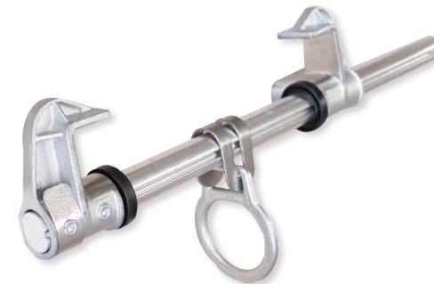
1702 Adjustable sliding beam anchor Fits flanges 3 1/2" to 14" wide, up to 1 1/4" thick Usable on top or bottom of I-beam Floating D-Ring
